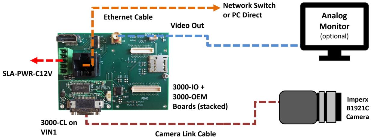
Figure 3: 3000-OEM Imperx Camera Bench Setup
