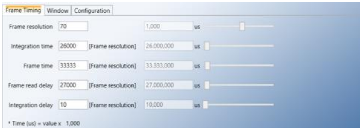
Figure 5: Example Frame Timing Settings (30 fps ITR Mode)
